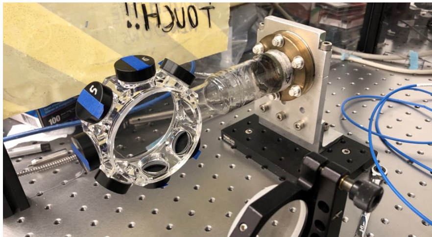
Figure 2.5: Nano-textured coated 3-inch octagonal glass cell.
