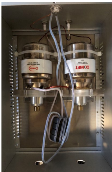
Figure F.2: (a) Tank circuit box used for each coil. Note the balancing variable capacitor is not shown in this photo. (b) 1kW RF amplifiers used for driving the RF MOT coils.
