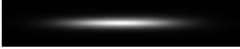
Figure A.8: A simulated phase-contrast image of 5 \times 10^6 atoms at 100 \mu\text{K} with a laser detuning of 60 MHz. Peak signal is 4.8I_o , and field of view is 2 mm by 0.4 mm.
