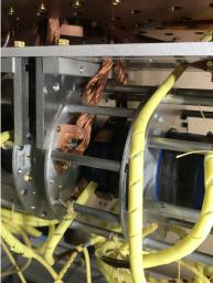
**Figure 3.6:** Images of the mounted magnets. On the left, a view of both magnets in the 4K cryogenic shielding, with optical access slits seen in the middle of each set. The blue packages are quench protection diodes, which were removed for the experiments described in the text. On the right, a close-up of the inner wall of one of the magnets, showing the copper braids bolted to the inside face. These braids were also clamped to the 4K stage of the pulse tube to cool the magnets.
