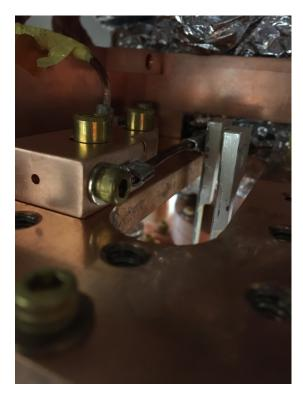
**Figure 3.7:** Picture of the electrical connection between the regular conducting lead (top left) to the HTS lead (silver, to the right). The block which they are connected through also serves as a heatsink, and is tightly clamped to the 40K shield through a sheet of kapton (not visible).
