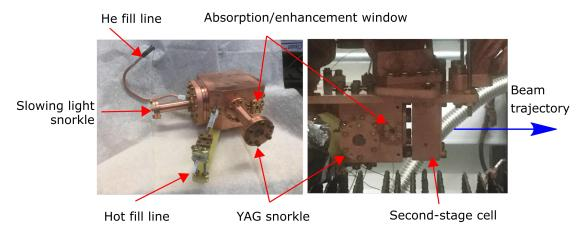
**Figure 4.3:** Picture of the cryogenic buffer gas beam cell. On the left is an assembled, but not mounted cell on which you can see several key components. On the right, the cell is mounted in the beam box, in the orientation we use experimentally.
