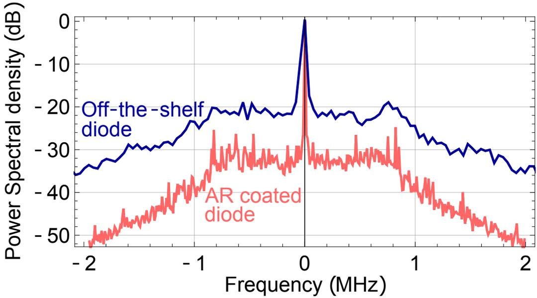
Figure 3.2.6: **Power spectral densities of the 690 nm STIRAP pump lasers.** The power spectral densities are typical of stabilized ECDLs with a very narrow central component on top of a much weaker broad pedestal. The AR-coated diodes provide a 10 dB reduction in the noise pedestal compared to the off-the-shelf diodes.
