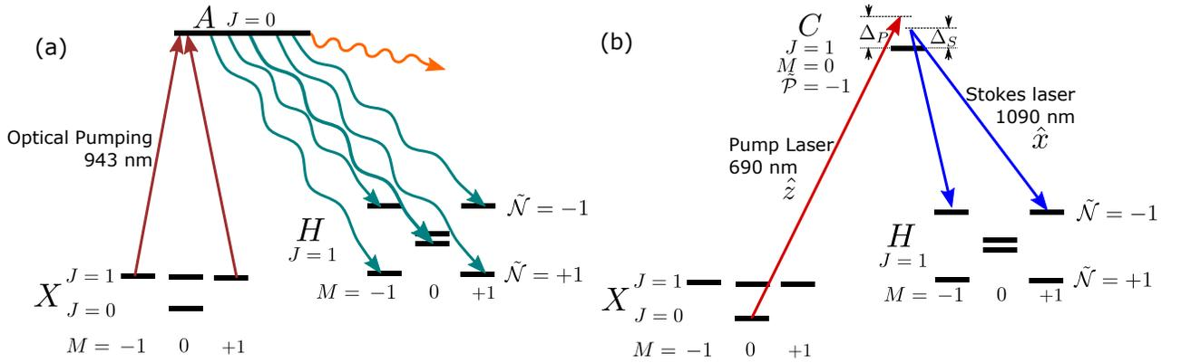
Figure 3.2.1: **Preparation of the initial spin-aligned state in  $H^3\Delta_1$ .** The state can be populated using either (a) an optical pumping scheme, as used in ACME I, or (b) a STIRAP scheme, as used in ACME II. For comparison purposes, we alternate between the two methods by blocking the corresponding laser beams. The detunings of the STIRAP Stokes and Pump lasers are shown as  $\Delta_S$  and  $\Delta_P$ , respectively.
