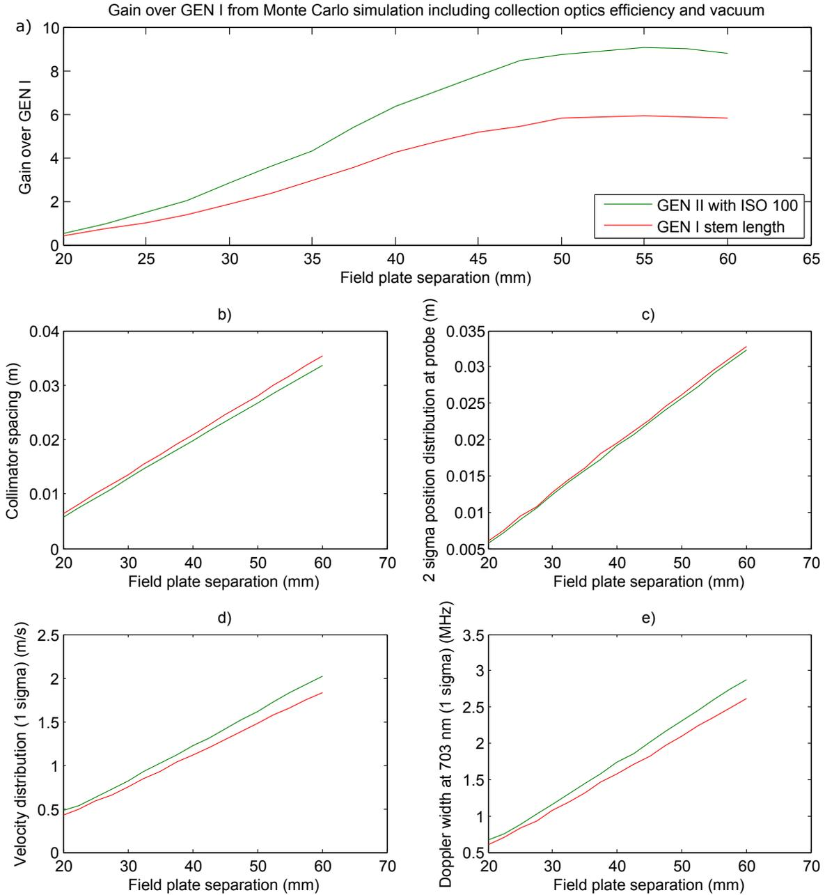
Figure 3.4.2: **Simulation data showing effects of increasing field plate separation on ThO beam properties.** All plots are shown for two different ThO beamline lengths: ACME I (red), and ACME II (green). The plots show: (a) signal gain over ACME I, (b) optimal collimator spacing, (c) size of the molecular cloud at the probe region, (d) the width of the velocity distribution and (e) its corresponding Doppler width at the probe wavelength of 703 nm.
