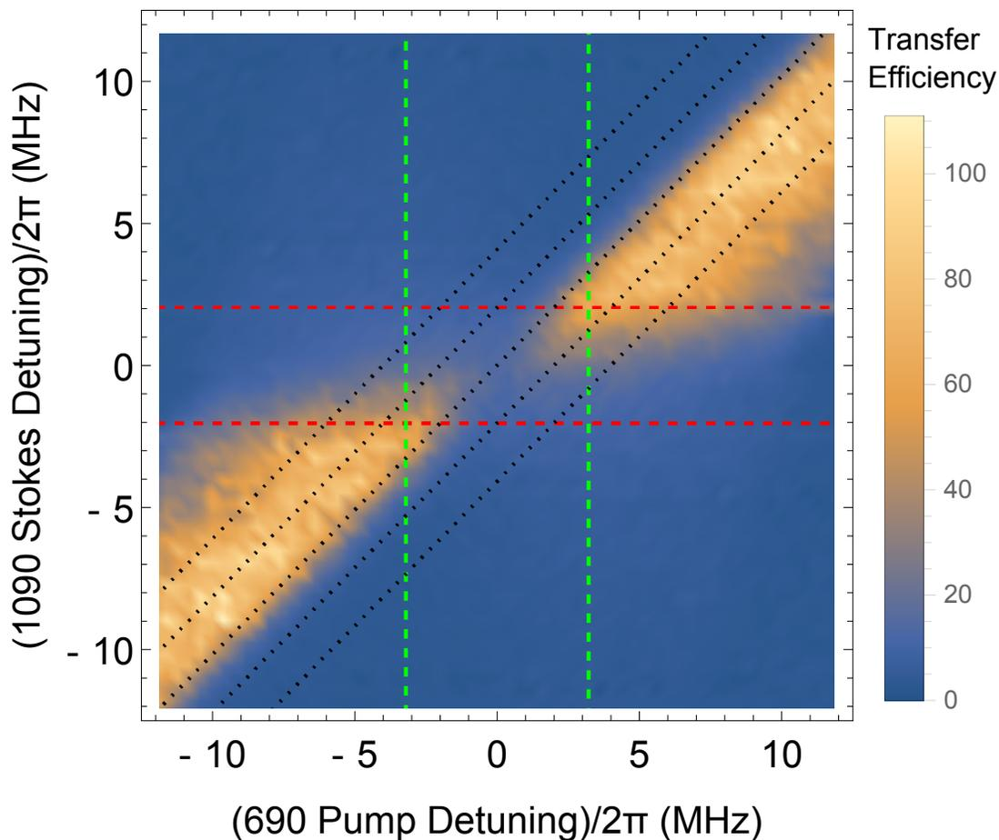
Figure 3.2.12: **Variation of STIRAP efficiency with detuning.** Density plot showing variation of the measured transfer efficiency with the detunings of the two lasers. Green (red) dashed lines are a guide to the eye, and indicate the extent of the pump (Stokes) one-photon resonance FWHM linewidth. Dotted black lines that indicate constant two-photon detunings are drawn at  $\delta \in 2\pi \times \{-4, -2, 0, +2, +4\}$  MHz.
