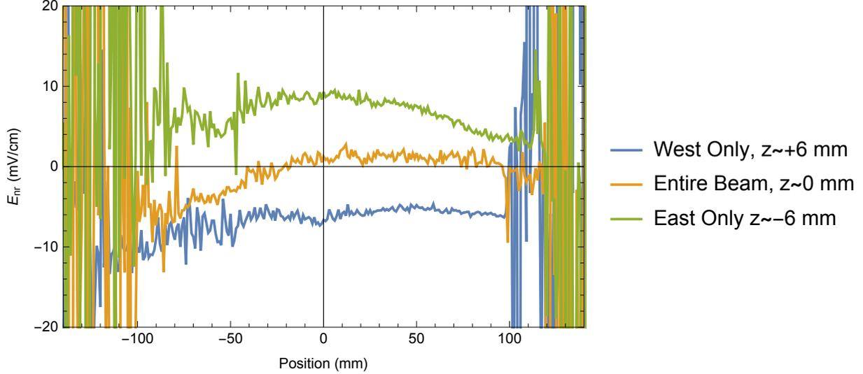
Figure 3.5.4: **Microwave measurement of  $\mathcal{E}^{\text{nr}}$ .** We measure the component of the electric field which does not reverse,  $\mathcal{E}^{\text{nr}}$ , at three different positions in the molecular beam along  $\hat{z}$ . This allows us to extract the gradients  $\partial\mathcal{E}^{\text{nr}}/\partial z$  and  $\partial\mathcal{E}^{\text{nr}}/\partial x$ .
