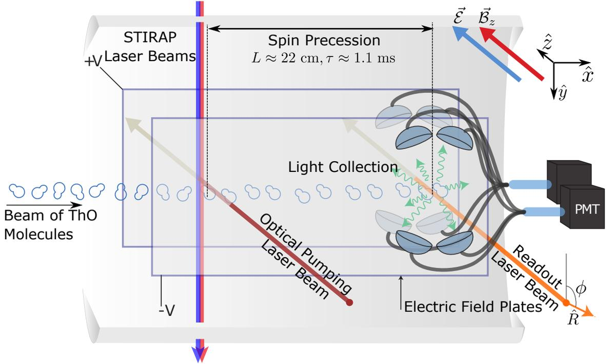
Figure 3.2.10: **Schematic of the experimental configuration used for implementing and testing STIRAP.** A collimated pulsed beam of ThO molecules enters the interaction region. The spin-aligned state is prepared, precesses in parallel electric and magnetic fields and is read out in the detection region by linearly polarized light, with resulting fluorescence collected and detected by photomultiplier tubes (PMTs).
