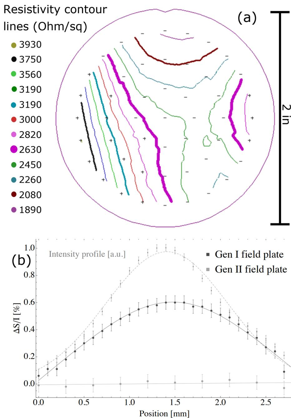
Figure 3.5.2: **Characterization of the ACME II field plates.** (a) Measured spatial variation in sheet resistivity of test glass pieces coated with a 20 nm thin layer of ITO. (b) Polarimeter measurement of the ellipticity gradient ( $\Delta S/I$ ) of the laser beam, after passing through the field plates. The light passing through the ACME II field plates shows significantly reduced birefringence gradient compared to ACME I.
