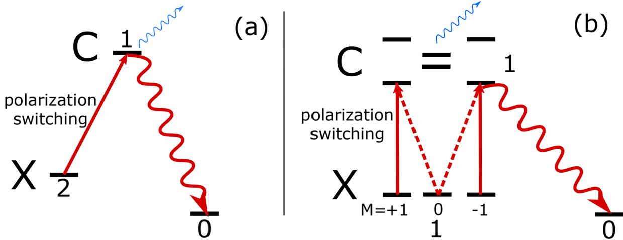
Figure 3.2.2: **The two ACME II rotational cooling steps.** (a) Population is transferred from  $|X, J = 2^+\rangle$  to  $|X, J = 0^+\rangle$  by optical pumping with 5–7 orthogonal polarization passes of a laser beam resonant with  $|X, J = 2^+\rangle - |C, J = 1^-\rangle$ . (b) An electric field mixes the parity of the  $|C, J = 1^\pm, M = \pm 1\rangle$  levels allowing for population to be transferred from  $|X, J = 1^-\rangle$  to  $|X, J = 0^+\rangle$ .
