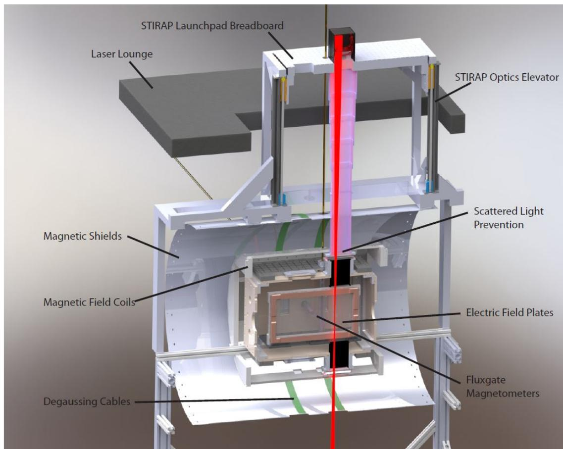
Figure 3.2.7: **Launching optics for the STIRAP lasers.** The optics are placed on a breadboard above the ACME II experimental apparatus. The STIRAP lasers are sent through the experiment vertically with a 45 degree mirror. A separately mounted platform (the “Laser Lounge”) allows personnel access for optics set up and alignment.
