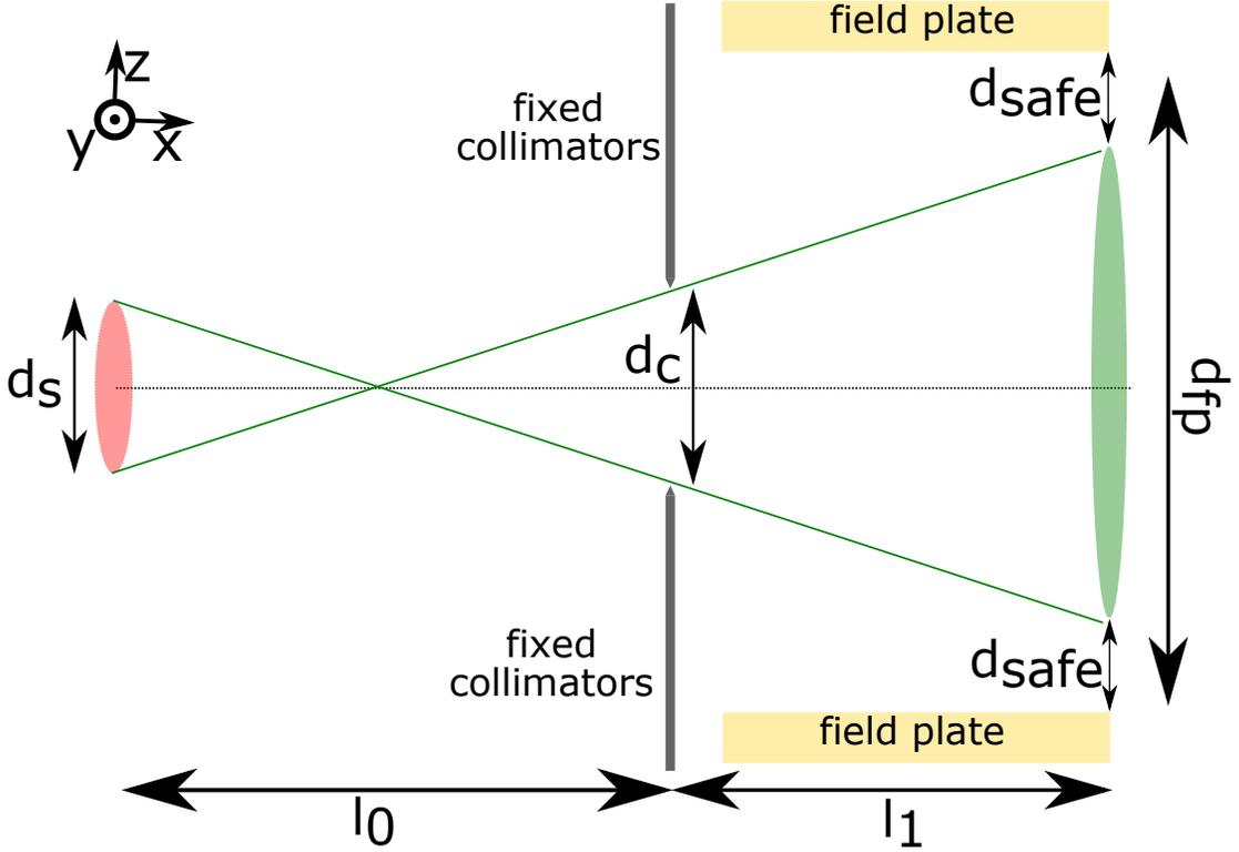
Figure 3.4.1: **Geometry of the ThO molecular beam.** The geometry is chosen such that there is no line of sight between molecules leaving the ThO molecular source of size  $d_s$  and the field plates. The size of the fixed collimators,  $d_c$ , is set by the separation between the electric field plates  $d_{fp}$ . An additional safety distance of  $d_{safe}$  accounts for missalignment in the system. Scales exaggerated for clarity.
