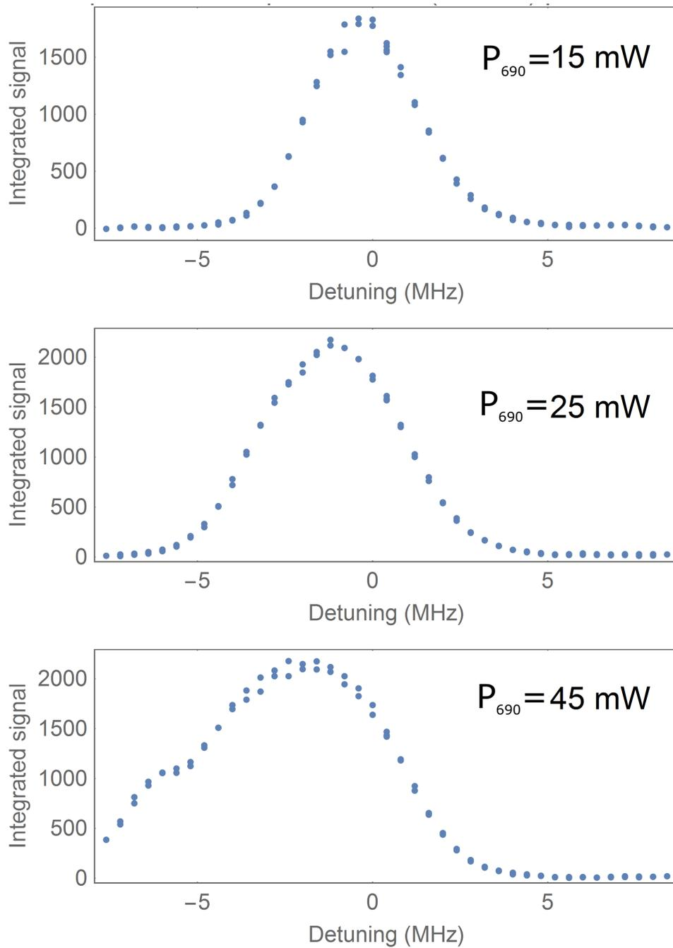
Figure 3.2.13: **Variation of STIRAP lineshape with 690 nm pump laser power.** As expected, the lineshape is symmetric when  $\Omega_S = \Omega_P$  and becomes more and more asymmetric as  $\Omega_P/\Omega_S \gg 1$ .
