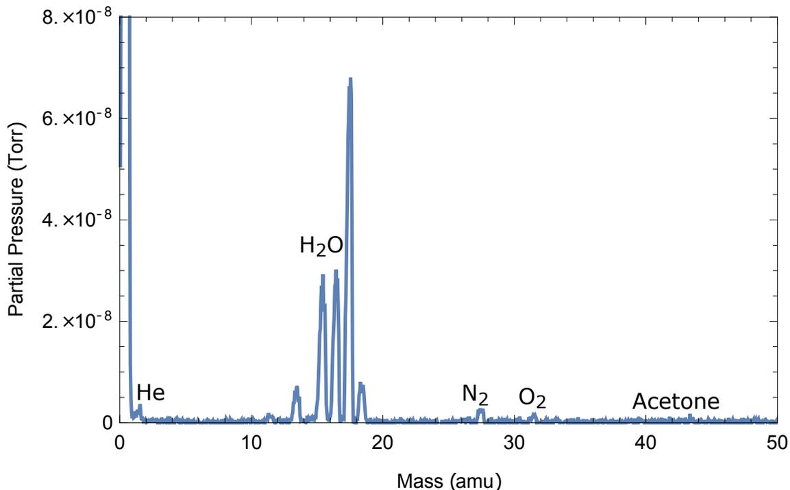
Figure 3.5.5: **Composition of the interaction region vacuum.** The composition of the interaction region vacuum after baking was measured with a residual gas analyzer (RGA). The largest peaks are due to water.
