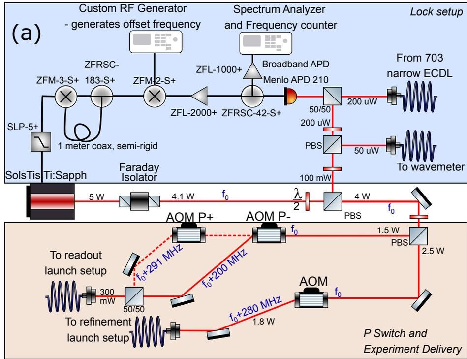
Figure 3.3.5: **Ti:S laser setup and fast frequency scanning.** (a) Optics for the Ti:S laser are used for locking (light blue background) or for performing the  $\tilde{P}$  switch and experiment delivery (light orange background). (b) Beat note measurement showing a Ti:S frequency chirp of 200 MHz in 5 ms, faster than that required for performing the  $\tilde{N}$  switch, which occurs every 0.6 ms.
