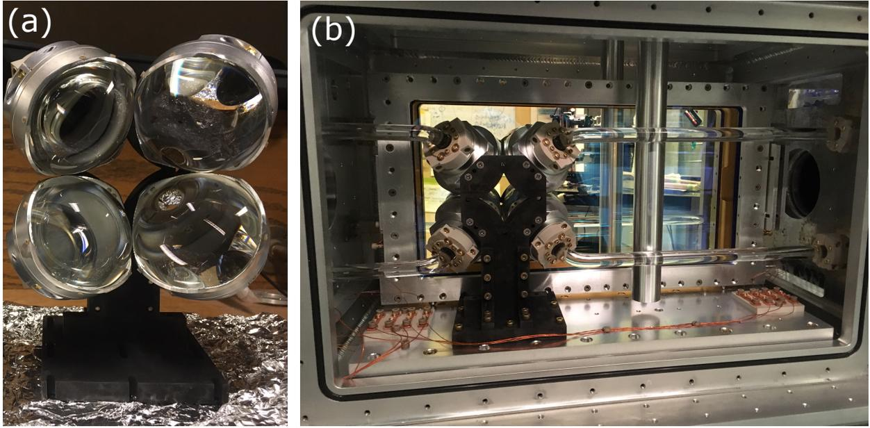
Figure 3.3.1: **ACME II collection optics.** (a) Front view of the 4 sets of lens doublets on one side of the experiment. They are mounted closely-packed on a rigid structure, such that the subtended fluorescence photon collection solid angle is maximized. (b) View of the inside of the interaction region, with collection optics installed. Glass lightpipes collect and transfer fluorescence light outside of the experiment chamber to the PMTs.
