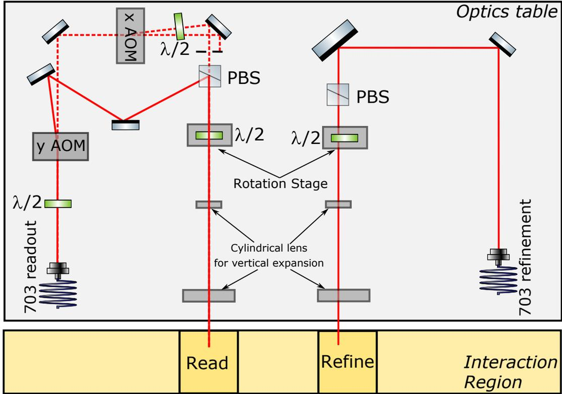
Figure 3.3.6: **Optical elements that deliver the 703 nm Ti:S light to the ACME II experiment.** Optics performing shaping of the laser beam spatial intensity profile, shown for both refinement of the readout laser beams. In addition, we use AOMs to quickly switch the polarization of the readout beam between orthogonal orientations,  $\hat{X}$  and  $\hat{Y}$ . The two beams are recombined on a high extinction ratio PBS before entering the interaction region vacuum chamber.
