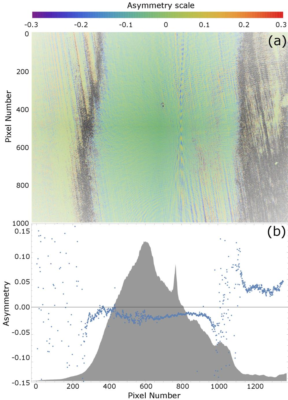
Figure A.1.1: **Measurement of linear polarization gradients in the refinement laser beam.** (a) Top figure shows the computed asymmetry between  $\tilde{\theta} = \pm 1$  states for the entire  $1360 \times 1024$  camera image. (b) The bottom figure shows the asymmetry as a function of  $x$  (horizontal) pixel number. The spatial intensity profile of the laser light along  $x$  during these measurements is shown in gray in the background.
