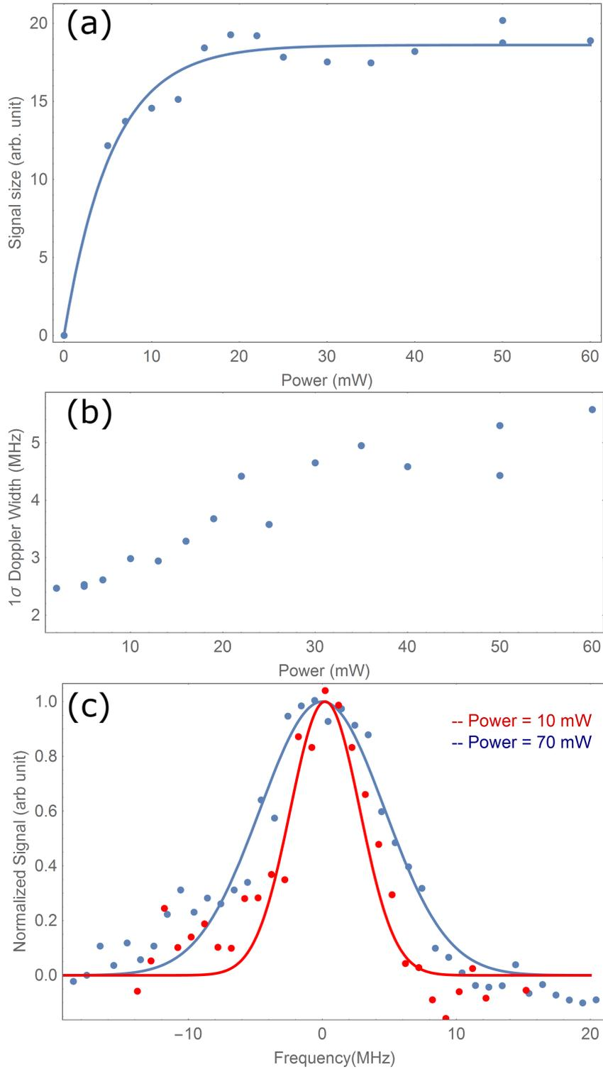
Figure 3.5.1: **Power saturation of the ACME II molecular beam.** (a) Signal size as a function of readout laser power. (b) Linewidth as a function of readout laser power. (c) Power broadened lineshape shown at 10 mW and 70 mW of power.
