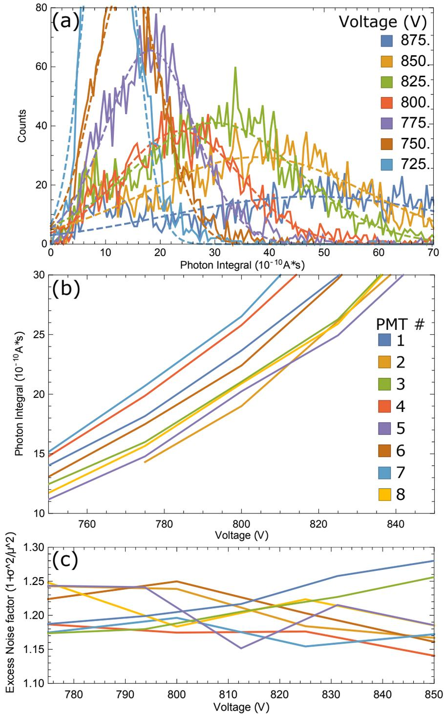
Figure 3.3.7: **Measurement of the PMT amplification factor.** (a) For a single PMT, histograms of the distribution of the integral below single photon pulses, for a number of applied bias voltages. For each of the eight PMTs, (b) variation of photon integral with applied bias voltage and (c) variation of the excess noise factor with voltage. The shown legend is common to plots (b) and (c).
