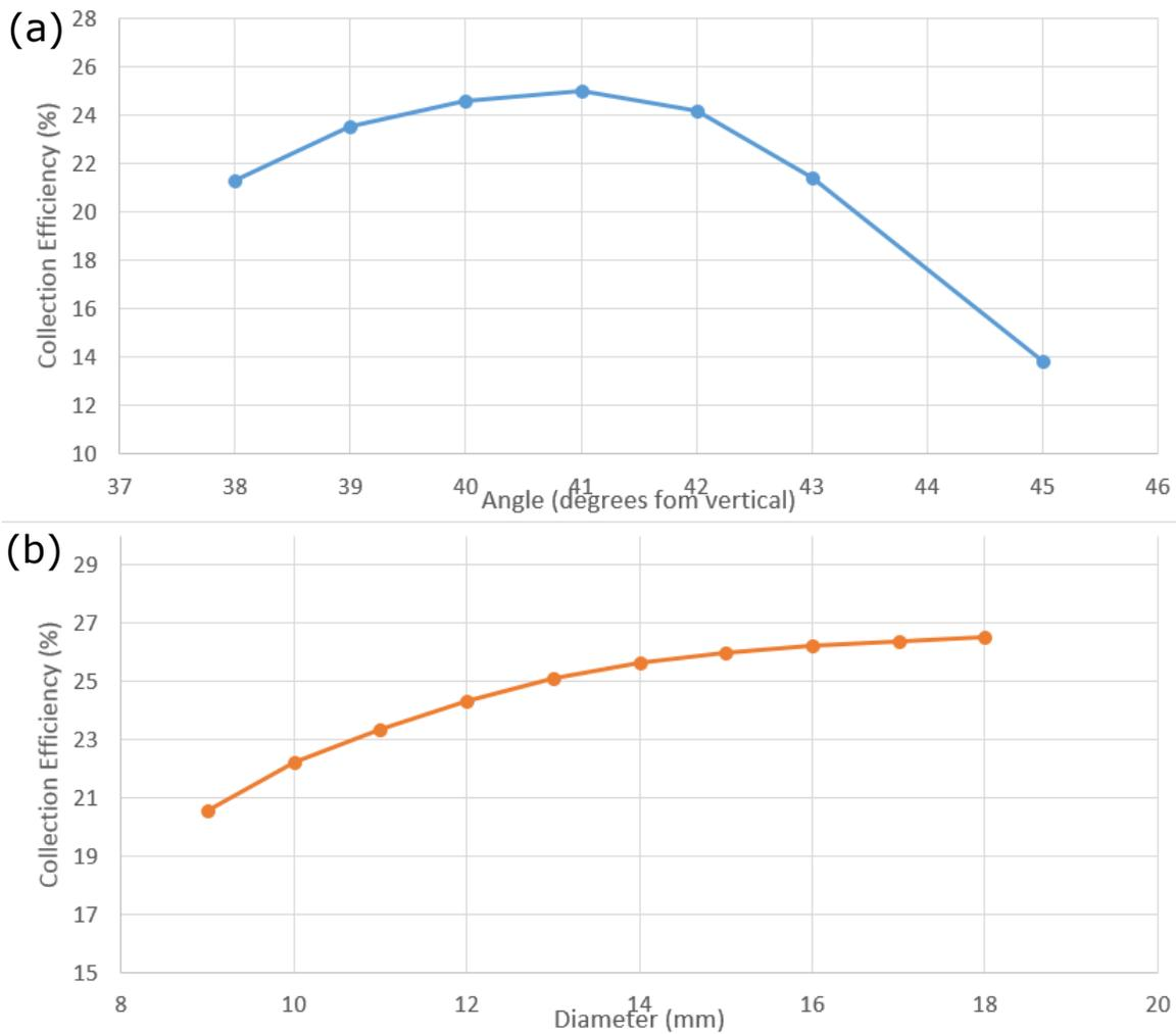
Figure 3.3.2: **Simulations of collection efficiency versus experiment geometry parameters.** (a) Efficiency versus angle of the collection lenses plane with respect to the vertical. An angle of 41 degrees is found to be optimal. (b) Recovery of collection efficiency with larger lightpipe diameters. Our lightpipe diameter (16 mm) recovers most of the gain loss when using the same diameter as was previously used in ACME I (9 mm) with the new geometry of our molecular beam.
