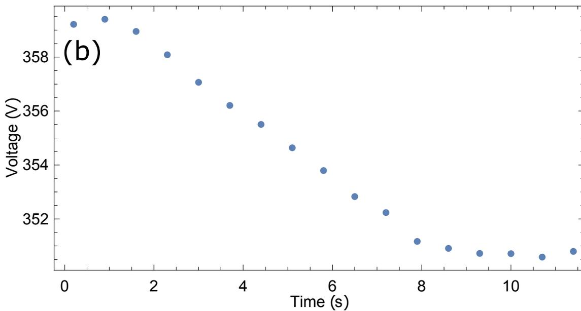
Figure 5.8.2: **Measurement of the leakage current.** (a) Calibration of the measurement lineshape, showing normalized molecular signal as a function of detuning due to the Stark shift caused by the electric field being away from the nominal 80 V/cm value. (b) Measurement of leakage current performed by measuring the decrease in signal over time, recalibrated using (a) to show decrease in voltage over time.
