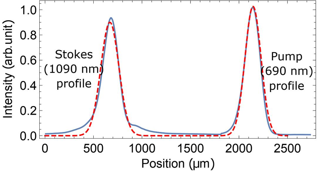
Figure 3.2.9: **STIRAP laser intensity profiles.** Typical normalized laser spatial intensity profiles (along the  $\hat{x}$  axis) at the center of the molecular beam (integrated over a 5 mm range along  $\hat{z}$  - blue line) and Gaussian fits (dashed red line). The beam profiles are greatly separated for clarity.
