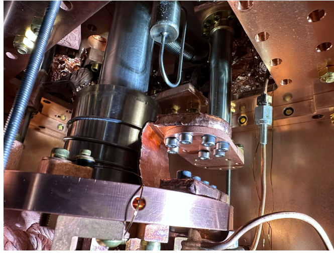
Figure A.4: Thermal switch that needed to be flipped upside down because Cryomech installed it in the wrong direction.
