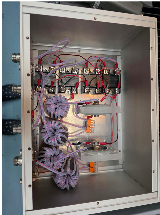
Figure 3.12: Components inside the DC circuit box.
