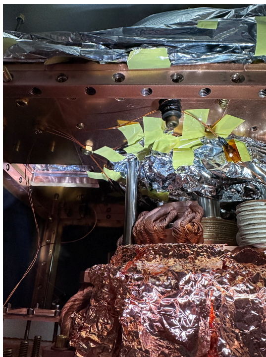
Figure A.8: Copper barrel used for heat sinking thermometer wires to the 40K shield. The wire is wrapped around and then covered with Stycast.
